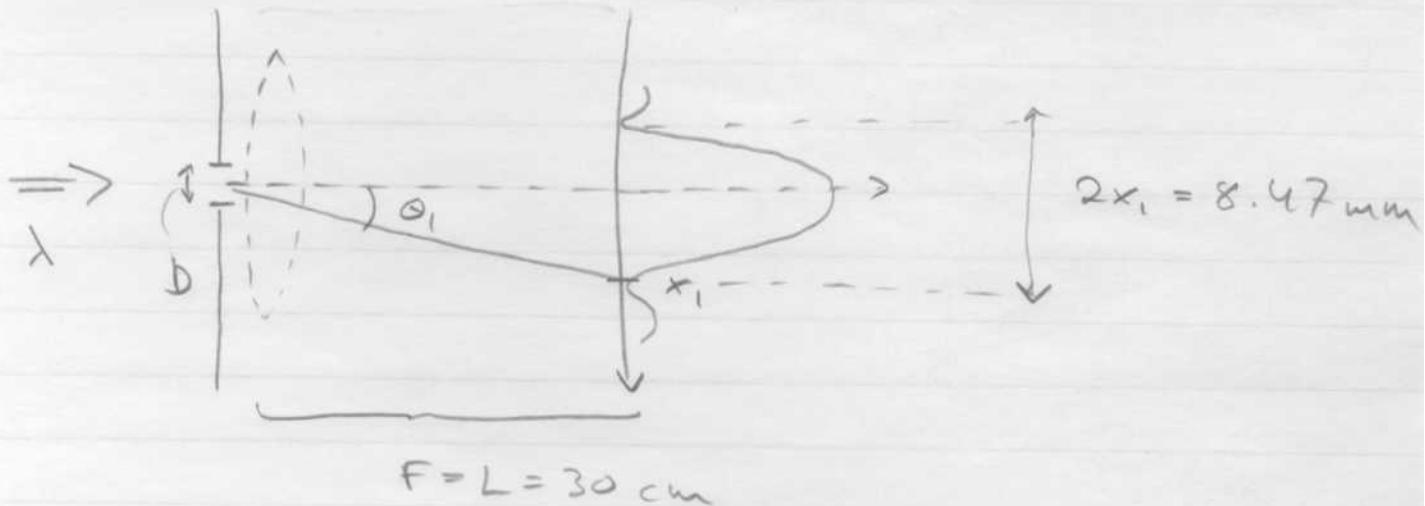
Med lins : Fraunhofer diffraction !
