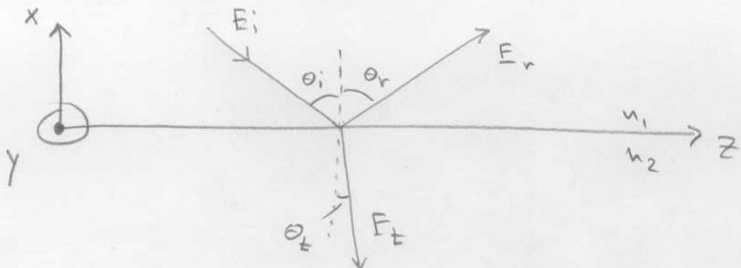
$$\left\{ \begin{array}{l} E_i = E_{i0} \cdot e^{i(\vec{k} \cdot \vec{r} - \omega t)} \\ E_r = E_{r0} \cdot e^{i(\vec{k}_r \cdot \vec{r} - \omega_r t)} \\ E_t = E_{t0} \cdot e^{i(\vec{k}_t \cdot \vec{r} - \omega_t t)} \end{array} \right.$$
