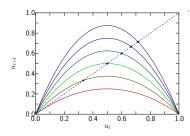
Curves for  $r = 1, 1.5, \dots 3.5$ . The solid dots show the respective steady state solutions,  $u_2^*$ .
