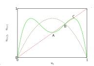
This phenomenon—which is here seen as a change from a simple steady state to an oscillation between two different values—is called a *bifurcation*.
