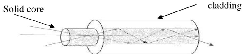
**Figure 1:** A typical conventional optical fiber
