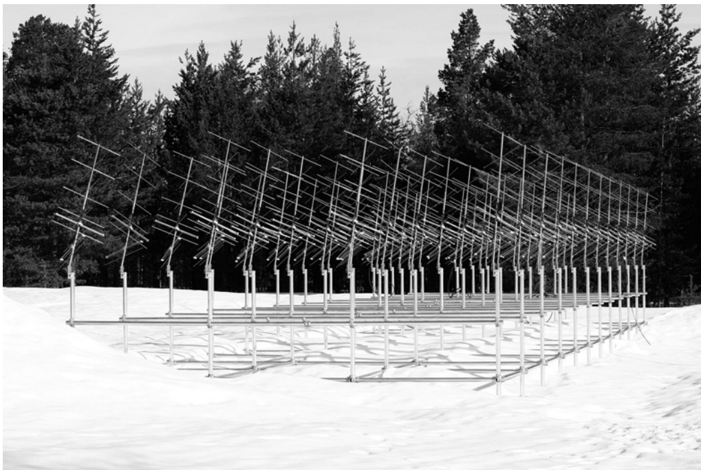
Figure 12.15.: The EISCAT_3D demonstrator phased array in Kiruna. This antenna has received signals from the VHF transmitter in Tromsø. Credits: EISCAT
